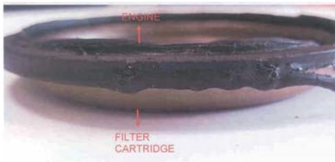
The investigation discovered that the gasket on the engine's oil filter converter plate had failed, allowing oil to flow out and causing the symptoms. It found that the maintenance organisation had mistakenly concluded that an FAA AD which called for the gasket to be replaced every 50 hours was no longer applicable.
